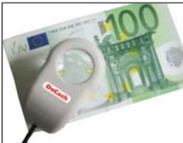
View of the image through 10x magnifier in visible range, with the possibility of backlighting.
